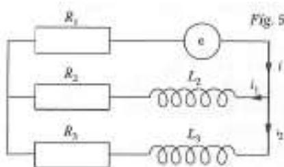
$$\begin{aligned} R_1 &= 30\Omega ; R_2 = 10\Omega ; R_3 = 20\Omega \\ L_2 &= 2\text{H} ; L_3 = 4\text{H} \end{aligned}$$
